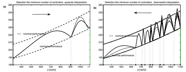
Figure 6: By upwards interpolation, (a), we need 3 controllers to cover  $\Pi$  and by downwards interpolation, (b), we need 10. Thin lines shows bisection procedure and thick line the final performance.
