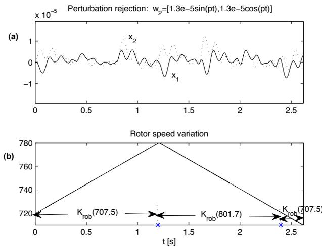
Figure 7: Simulation in closed loop. The scheduled parameter increases within 1.2 sec from 720 to 780, and decreases back to 710 within another 1.5 sec. Three controllers  $K_{\text{rob}}(p(t))$  are called for. Upper image shows unbalance compensation  $x_1, x_2$  for simulated  $w_2(t) = (1.3e - 5 \sin p(t), 1.3e - 5 \cos p(t))$ . (For  $x_1, x_2, w_2$  see section 2).
