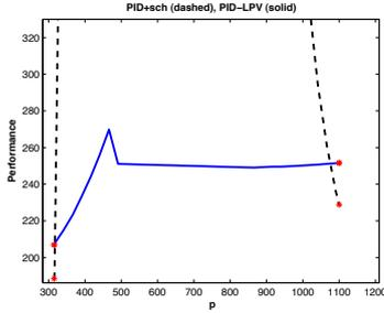
Figure 4: Interpolating linearly between the two controllers  $K^*(315)$  and  $K^*(1100)$  (dashed line) fails due to a loss of stability, while switching using  $K_{\text{rob}}(315)$  and  $K_{\text{rob}}(1100)$  holds the stability (solid line).
