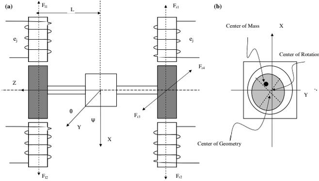
Figure 1: Left image, (a), shows the magnetic bearing configuration with magnetic forces  $F_{r1}, \dots, F_{r4}, F_{l1}, \dots, F_{l4}$  according to (R.D. Smith, 1995). Right image, (b), shows the rotor unbalance. The purpose of unbalance compensation is to drive the displacements  $x_1 = L\theta$  and  $x_2 = L\psi$  to 0.
