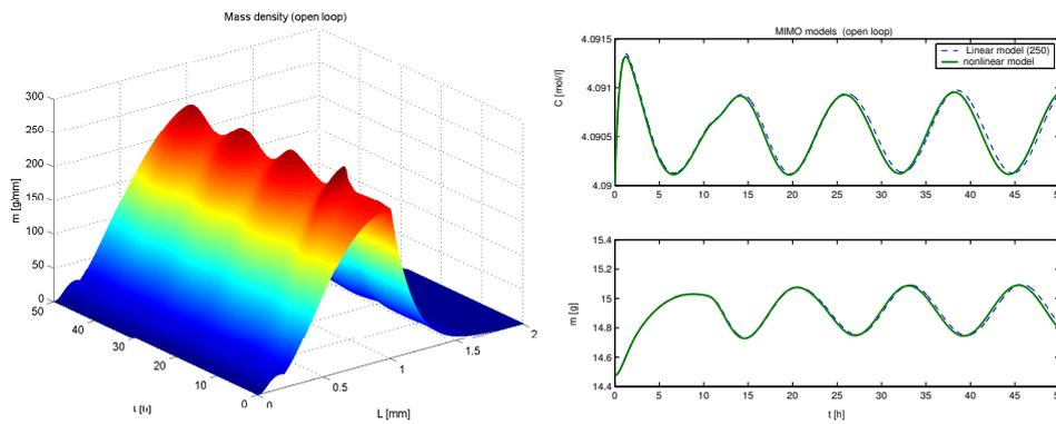
Figure 37.1: Sustained oscillations of slurry rate and solute in open loop.
